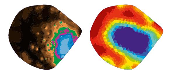
Sonic tomogram (left) and electrical resistance tomogram (right) of a lime tree with cavity and rot
